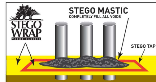
FIGURE 5: MULTIPLE PIPE PENETRATION SEALING
