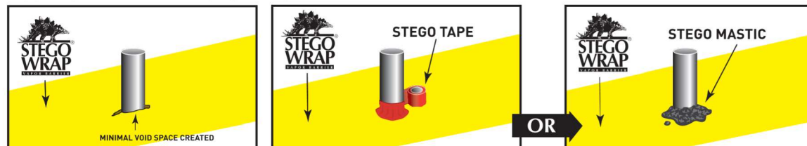
FIGURE 4a: PIPE PENETRATION SEALING
